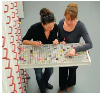
Picture 4. Radix Polaris: two freezing aisles in a cool room. Each aisle consists of twelve sections of one cubic metre each. The resulting 24 m 3 storage space replaces 36 conventional ultrafreezers.
